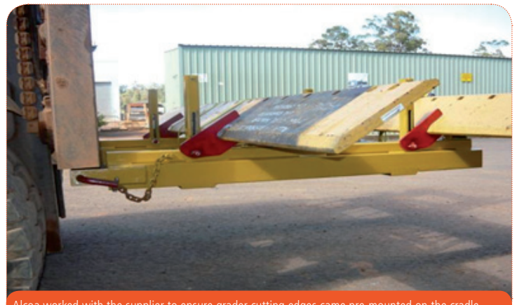
Alcoa worked with the supplier to ensure grader cutting edges came pre-mounted on the cradle
