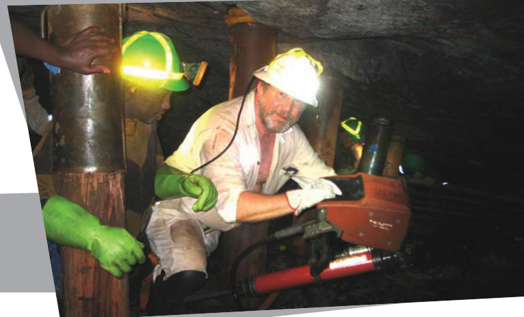
The leader of the Noise Adoption Team tries out the electric rock drill identified by his team as a leading practice for reducing noise induced hearing loss.
